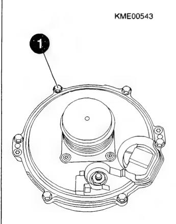
ASSEMBLING ALTERNATOR Alternator leak test Fit nut (1) of B+ connecting cable (Boellhoff nut). Use torque wrench. Tightening torque: 10,1...13,5 Nm Torque wrench: comm. avail.
